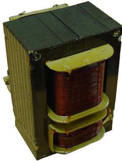
Figure 9.10: Example of a gas-discharge lighting transformer.
